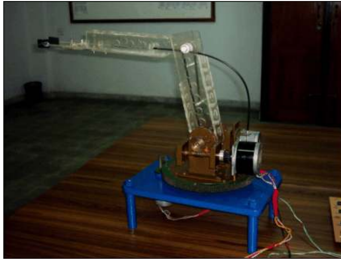
Fig. 1: Pick and Place Robot with Gripper Hand (Kabir et al. , 2003)
