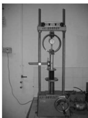
Fig. 1: Unconfined compression test using 4.5 kN ELE proving ring
