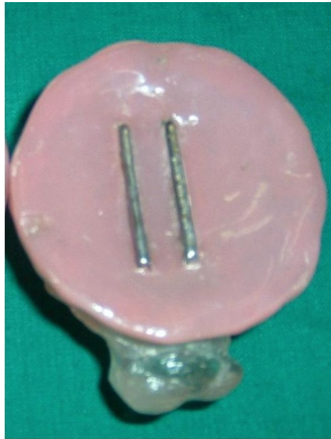
Fig. 7: The terminals of the carbon steel plates extending to the outer surface of the acrylic lid.
